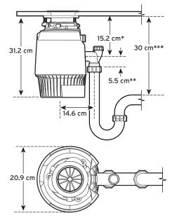
\*Distance from bottom of sink to centre line of disposer outlet. Add 12.7 mm when stainless steel sinks are used.
