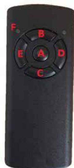
*Note : If the RC functions are limited or not available please check battery capacity first ( LED (F) ).*
